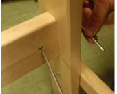
(\*) = sleeve nut + threaded rod + barrel nut Hammer the barrel nut in place. Set the position with a screwdriver.
