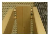
6. Set the wooden dowels (J) in the holes of the front legs and put the breast beam (5) in place. Do the same with the back legs and the back beam (6).
