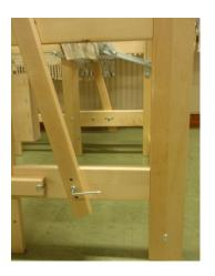
8. Remove the cotter pin from the treadle rod (24) and put the treadles (23) and the treadle spacers (I) in place. Lock the rod with the cotter pin.
