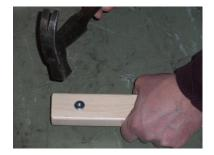
3. Fasten the lower front rail (3) and the lower back rail (4) on the right side of the loom (2) with 2 furniture bolts (D) 6x60 mm (= sleeve nut + threaded rod + barrel nut (\*)).
