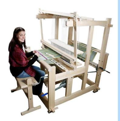
The large side opening allows for easy access to warp and tie-up.
